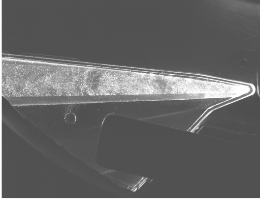
Fig. 2 Converging PIV light sheet with thickness tailoring.
